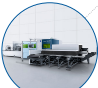
TRUMPF – TruLaser Tube Laser tube cutting machine
