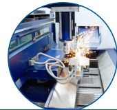
TRUMPF – TruLaser Cell 3D-Laser tube cutting machine
